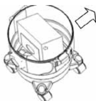
2. Take out the paper filter. *Paper filter OPCIONAL
